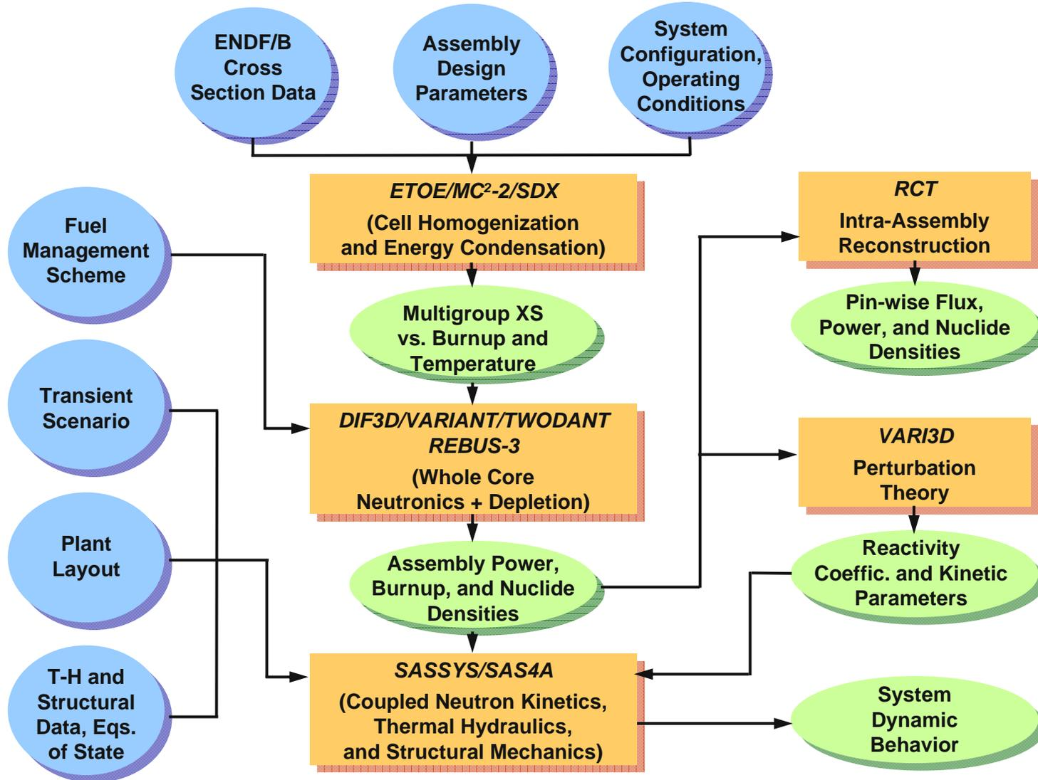
*This has evolved to a modern thermal hydraulics code (SHARP), coupled to neutronics ...*
